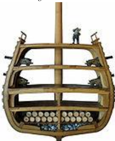
A model showing Vasa's hull cross section, illustrating the shallow keel and two gun decks.
